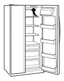
The temperature controls are preset in the factory at **5** for both the refrigerator and freezer compartments. Allow 24 hours for the temperature to stabilize to the preset recommended settings.
